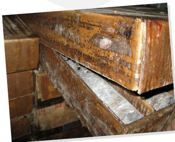
Coal-bed methane core in need of immediate curation.
