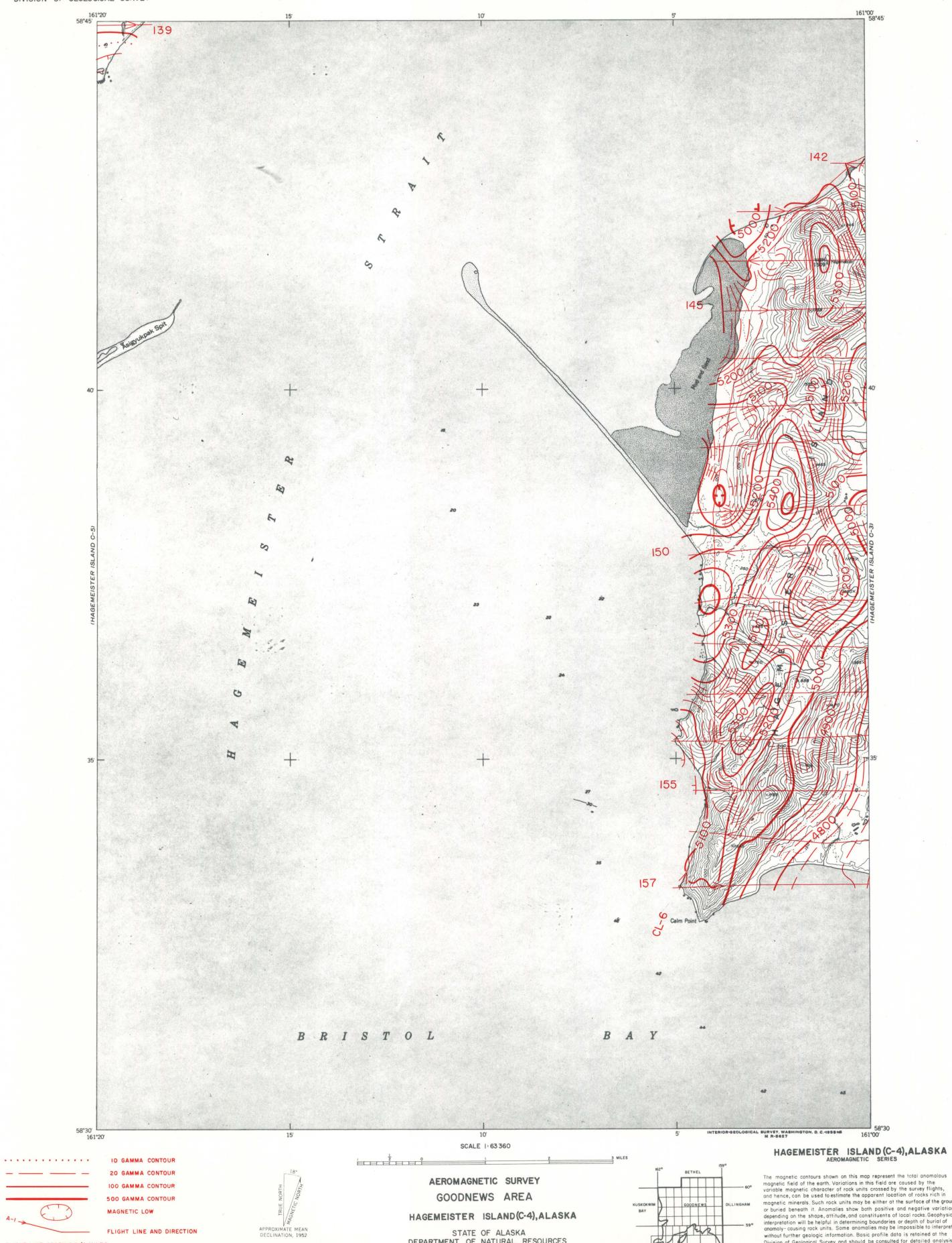
FLIGHT LINE SPACING 3/4 MILES FLIGHT ALTITUDE NOMINALLY 1000 FEET ABOVE GROUND REGIONAL MAGNETIC FIELD SW SHEET CORNER: 53,213 GAMMAS REGIONAL FIELD REMOVED. THE FIELD INCREASES APPROXIMATELY 7.0 GAMMAS/MILE, N 29°E APPROXIMATE FIELD INCLINATION: + 70.8°
