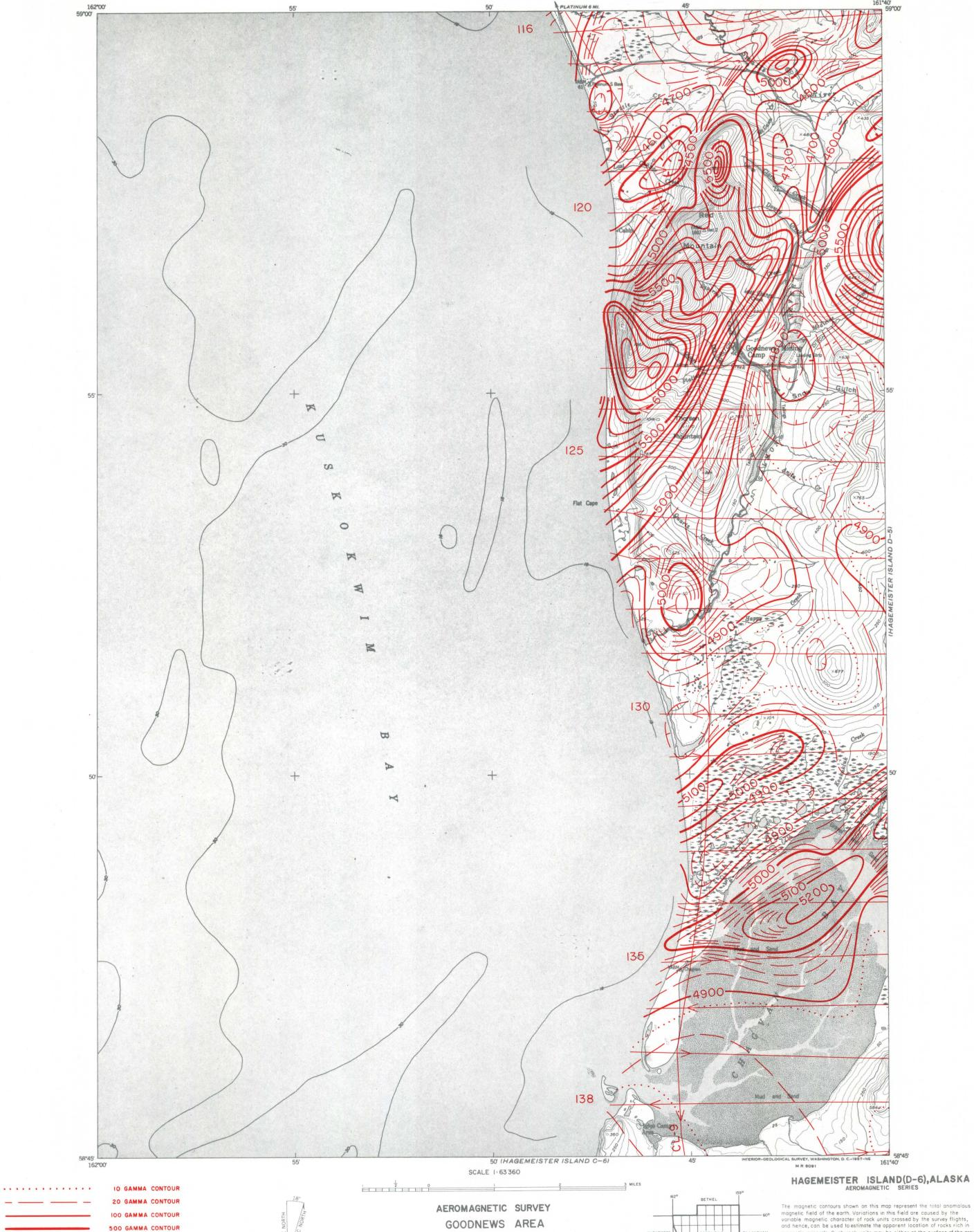
FLIGHT LINE AND DIRECTION FLIGHT LINE SPACING 3/4 MILES FLIGHT ALTITUDE NOMINALLY 1000 FEET ABOVE GROUND REGIONAL MAGNETIC FIELD SW SHEET CORNER: 53,243 GAMMAS REGIONAL FIELD REMOVED. THE FIELD INCREASES APPROXIMATELY 7.0 GAMMAS/MILE, N 29°E APPROXIMATE FIELD INCLINATION: + 70.8°
