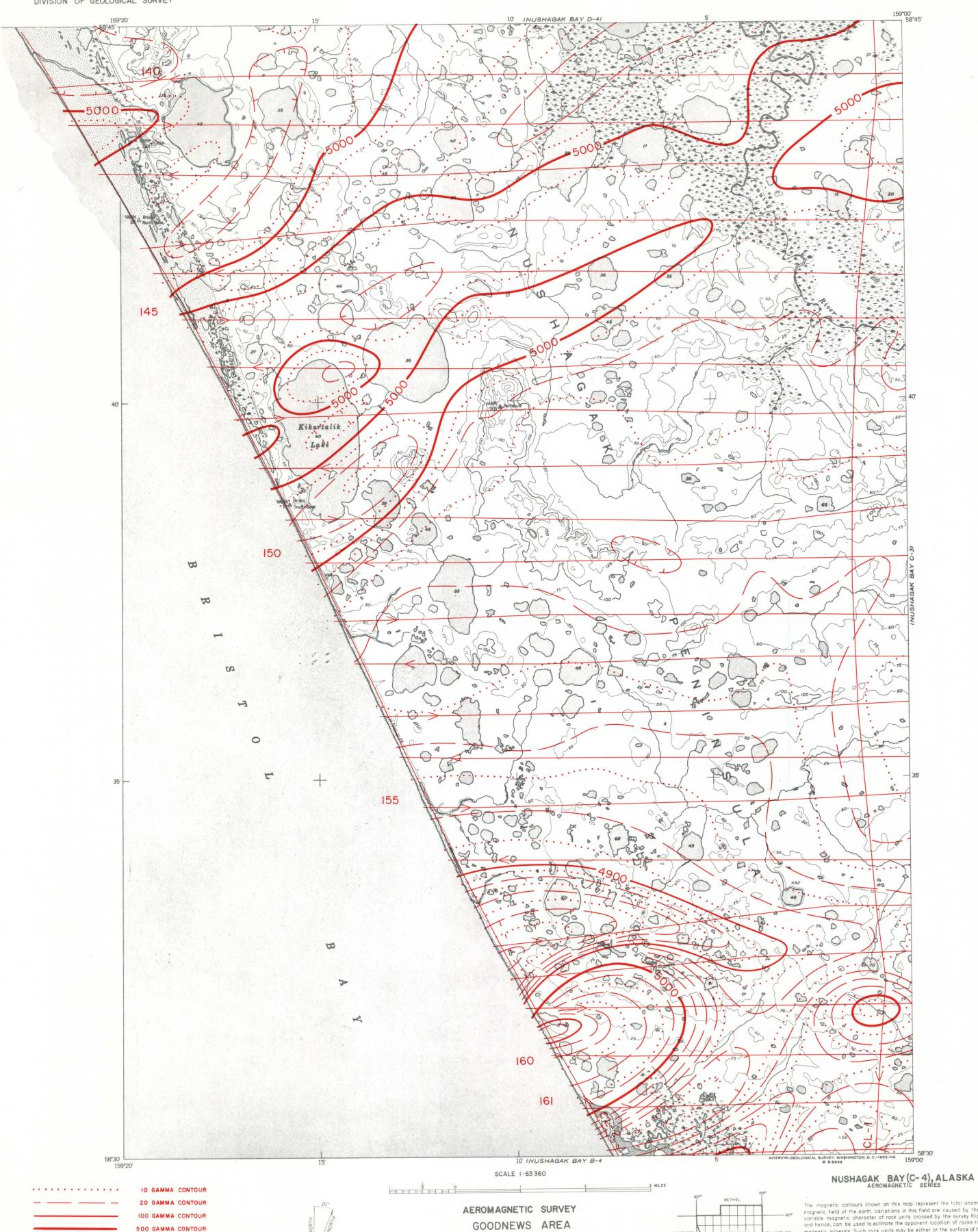
FLIGHT LINE SPACING 3/4 MILES FLIGHT ALTITUDE NOMINALLY 1000 FEET ABOVE GROUND REGIONAL MAGNETIC FIELD SW SHEET CORNER: 53,452 GAMMAS REGIONAL FIELD REMOVED. THE FIELD INCREASES APPROXIMATELY 7.0 GAMMAS/MILE, N 29° E
