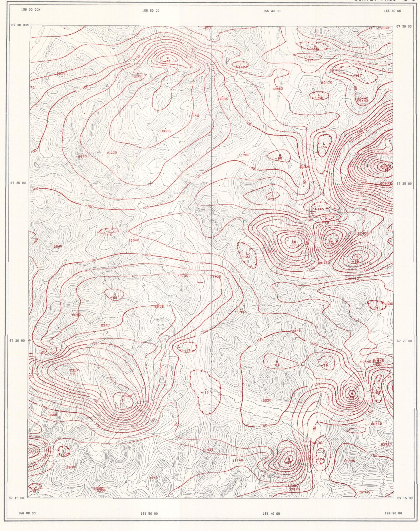
10.0 GAMMAS CONTOUR INTERVAL 56648.31 GAMMAS DATUM . 0.75 & 1.0 MILE(S) FLIGHT LINE SPACING FLIGHT ALTITUDE ..... 24°02' E MAGNETIC DECLINATION . 77°25' N MAGNETIC INCLINATION . FLOWN AND COMPILED 1975 INSTRUMENT. ... GEOMETRICS G-803 PROTON MAGNETOMETER
