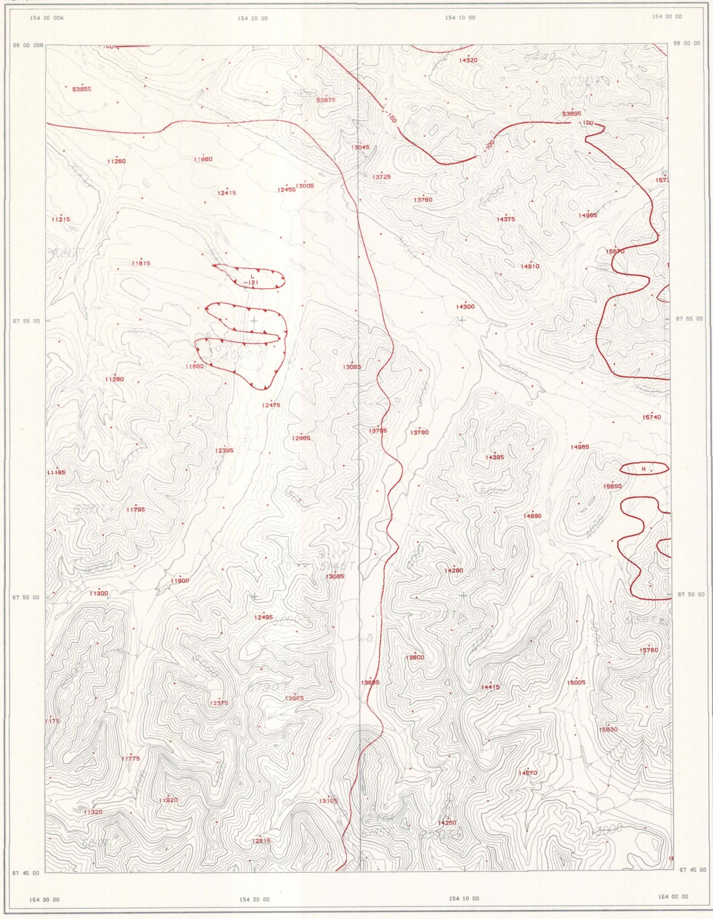
10.0 GAMMAS CONTOUR INTERVAL 56861.71 GAMMAS 0.75 & 1.0 MILE(S) FLIGHT LINE SPACING ... 1000 FEET AGL FLIGHT ALTITUDE MAGNETIC DECLINATION . MAGNETIC INCLINATION 77°57' N . . . . . . . . . . . . . . 1975 FLOWN AND COMPILED ... INSTRUMENT .... GEOMETRICS G-803 PROTON MAGNETOMETER
