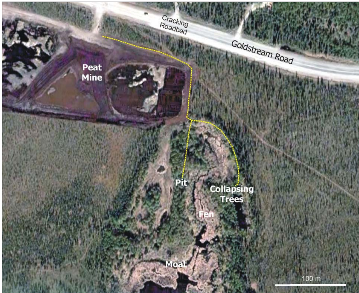
Figure 1. Southeast of the peat mine are thermokarst pits, fens, and actively collapsing forests. A “moat” surrounds the margins of areas with rapidly collapsing permafrost. After collapse, the groundwater-fed water body quickly becomes colonized by sedges and cattails to become a fen.
