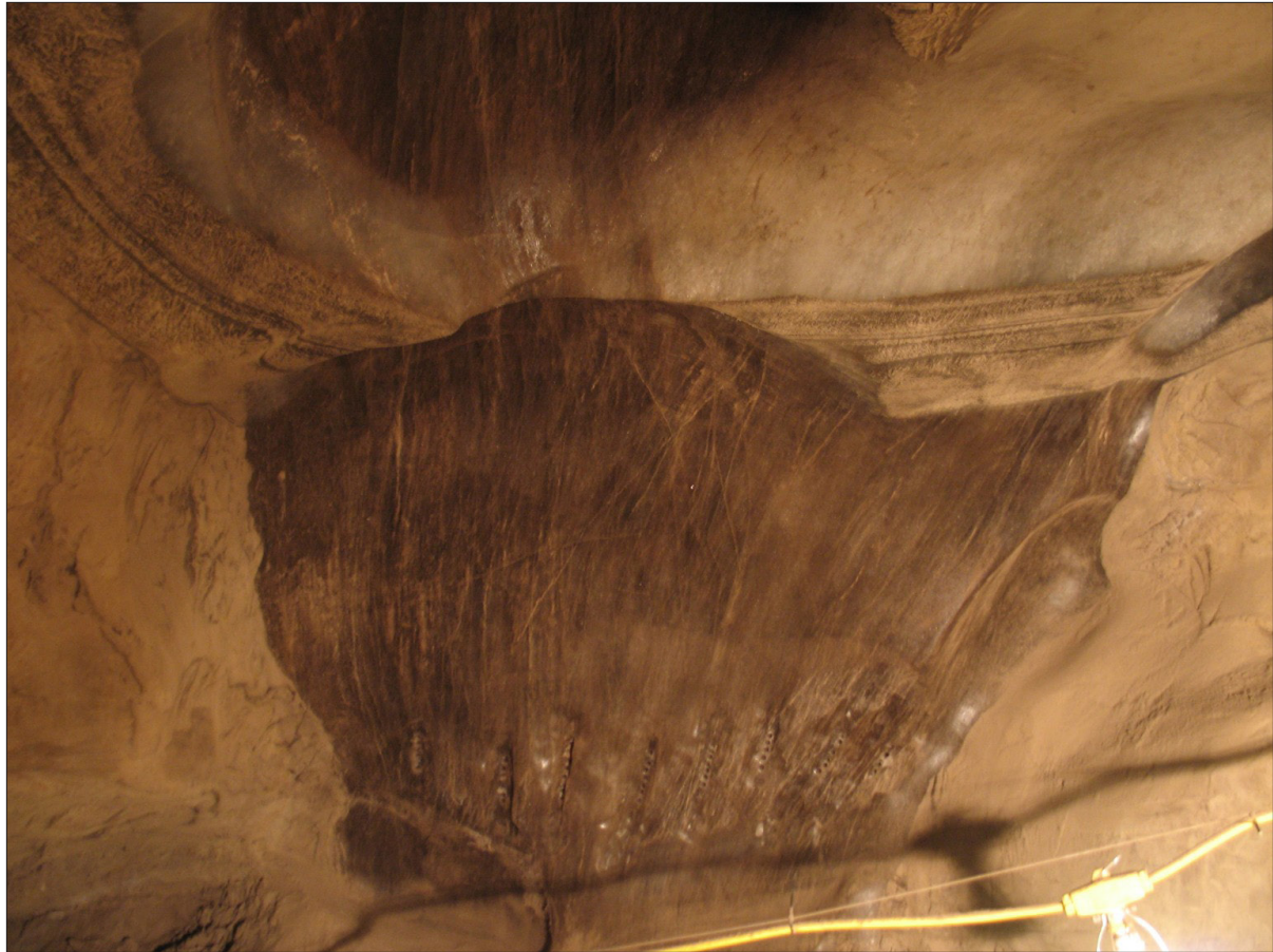
Figure 14. Photo showing ice wedge dissecting a horizontal lens of white thermokarst-cave ice (ice pseudomorph), right wall of the winze. The width of the wedge is 1 m. The thermokarst-cave ice body is underlain by several silt layers with reticulate-chaotic cryostructure. The same wedge exposed on the opposite wall of the winze is shown in figure 12. (Photo by M. Kanevskiy.)
