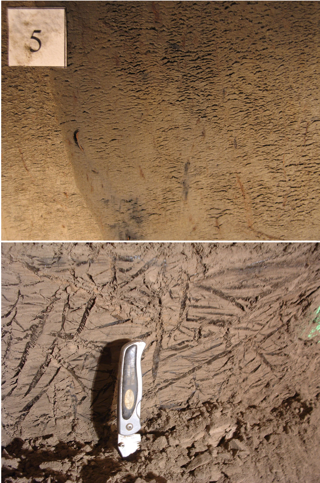
Figure 5. Photos showing (A) micro-lenticular cryostructure (location marker is 1.25 x 1.25 cm in size) (photo by M. Kanevskiy), and (B) reticulate-chaotic cryostructure (the handle of the knife is about 6 cm long) (Fortier and others, 2008).
