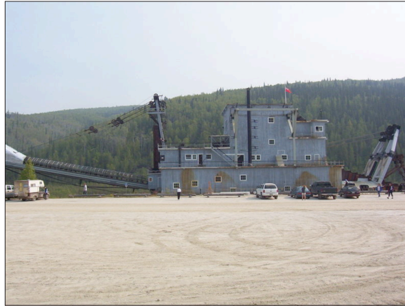
Figure 2. Example of gold-mining dredges used at Gold Hill. The gravel was taken into the dredge using the excavator buckets on the right. The gold was separated from the gravel in the dredge using mechanical and chemical processes, and the processed gravel was dumped behind the dredge by the large boom on the left.
