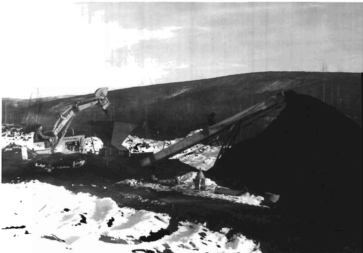
Fig.1. Mining and shredding peat at Pit No. 2, Alaska Resources, Inc.
