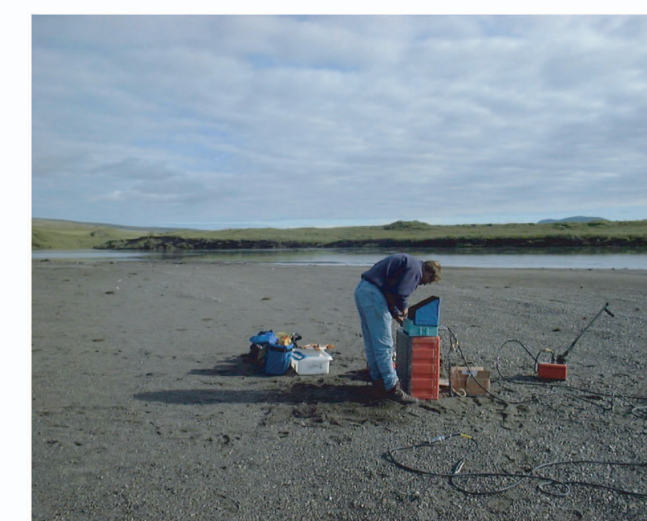
Figure 3. Operation of the GSSI System 2000 and 400 MHz transducer (right).
