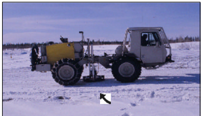
Figure 3. Articulated tractor-mounted mini-vibrator with hydraulic pad (arrow) used for generating compressional waves. Fort Yukon, April 2001.
