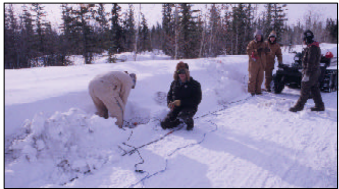
Figure 2. Seismic cable laying and geophone drilling on side of Fort Yukon road, April 2001.
