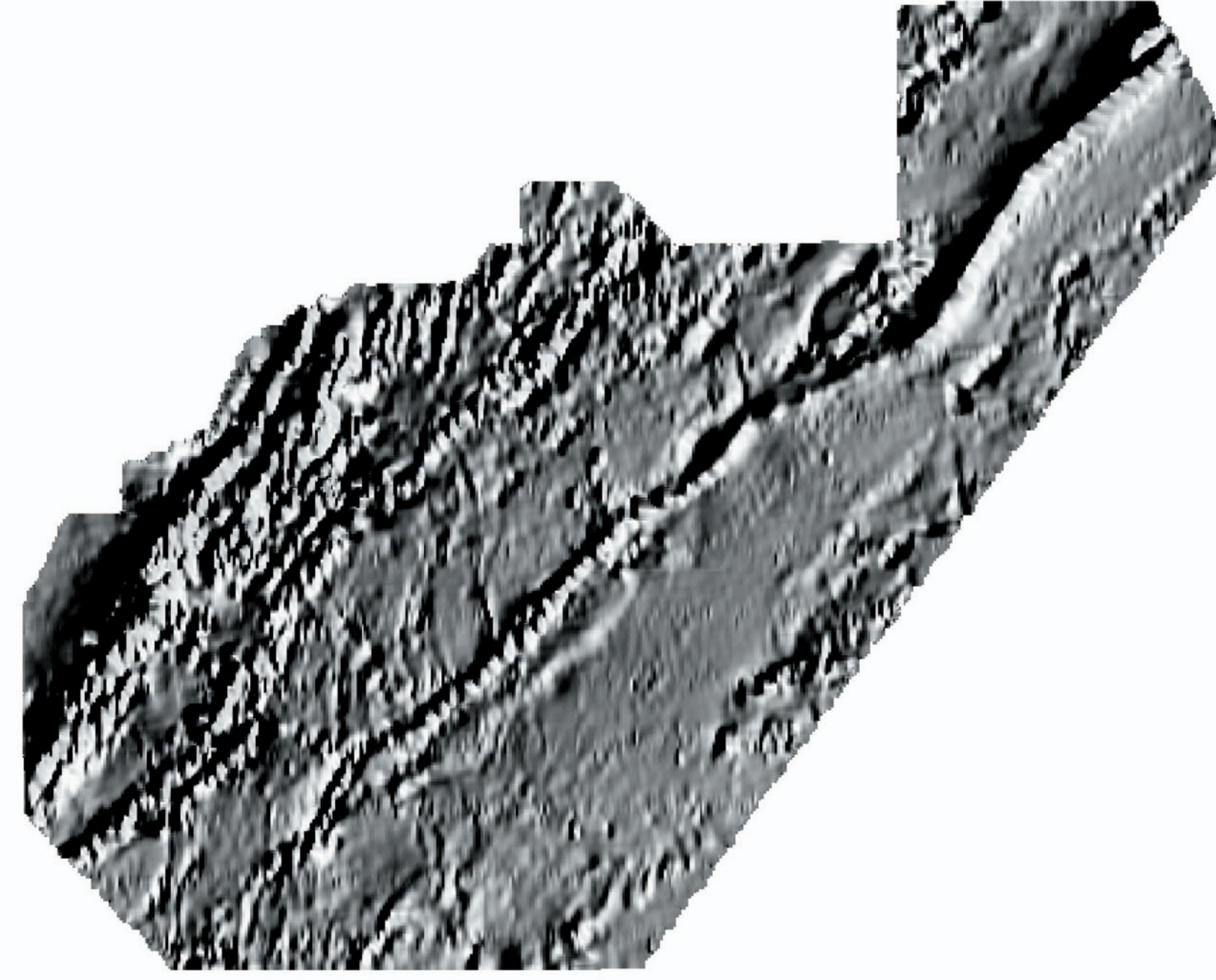
Figure 2: Shadow map of the aeromagnetic data from the Chulitna area, Alaska. Illumination source is at 111 degrees. High magnetic values appear like the tops of mountains that are hit by sunlight. This image emphasizes northeast and north trending structures.
