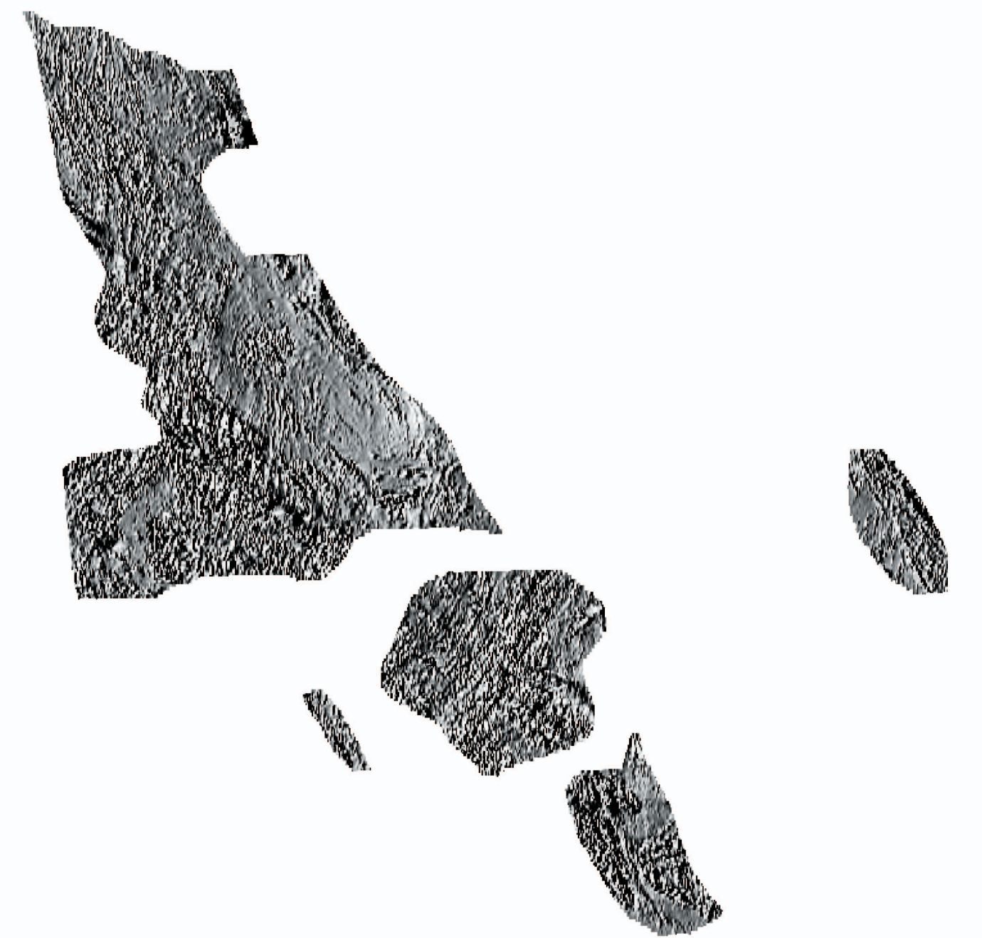
Figure 3: Shadow map of the aeromagnetic data from the Stikine area, Southeast Alaska. Illumination source is at 282 degrees. High magnetic values appear like the tops of mountains that are hit by sunlight.
