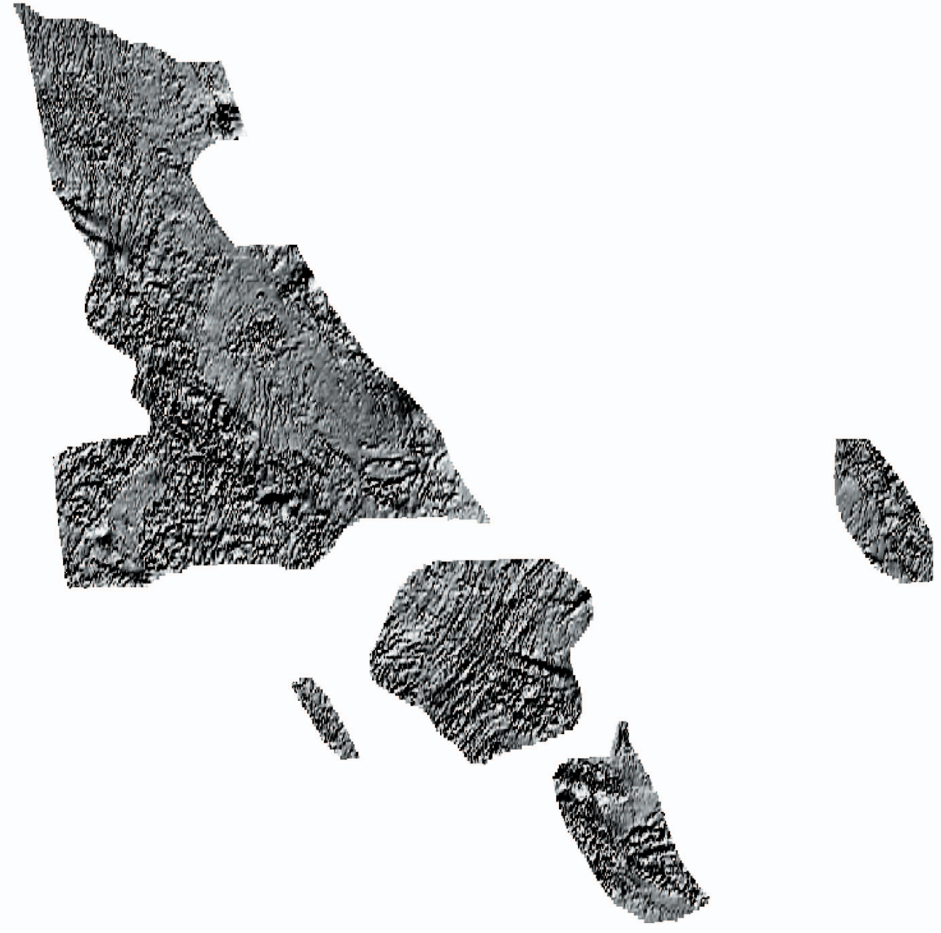
Figure 2: Shadow map of the aeromagnetic data from the Stikine area, Southeast Alaska. Illumination source is at 147 degrees. High magnetic values appear like the tops of mountains that are hit by sunlight.
