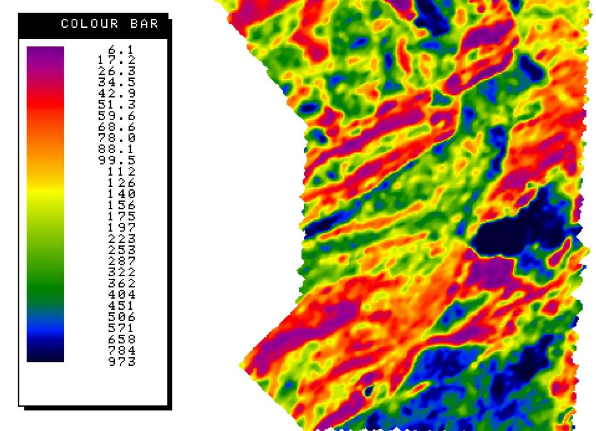
Figure 6: 7200 Hz resistivity map of the Ruby area. Resistivity values in ohm-m. Conductive units have low numbers and are shown in purple and orange on this map.
