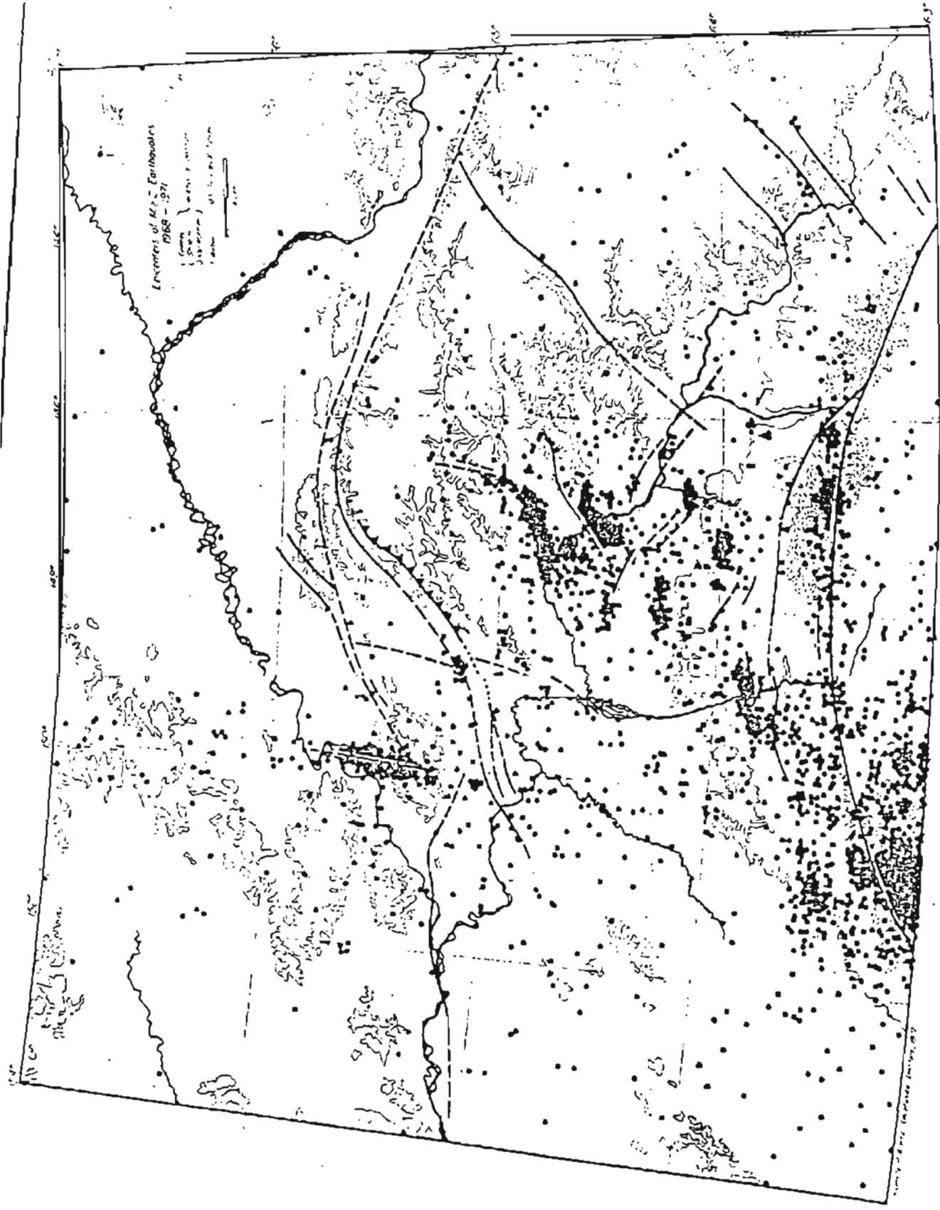
Figure 5: Correlation of epicenters with mapped faults. Note both ENE-WSW and NNW-SSE alignments of epicenters trending through the Fairbanks area. From Gedney and others (1972).
