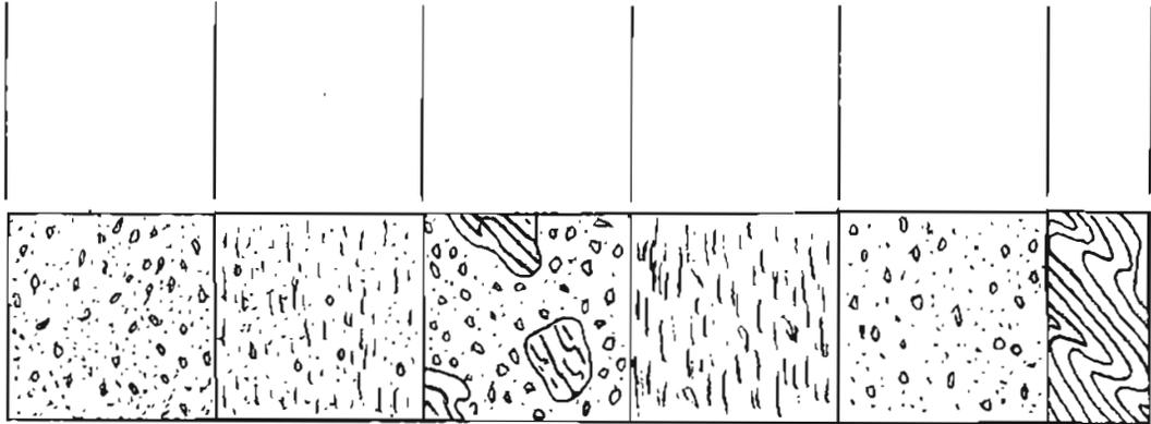
UNIT 1--Surficial fluvial sand and gravel deposit, 20 to 30 feet thick, thins to the west.
