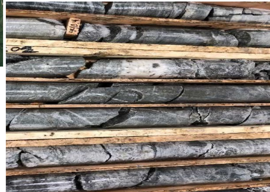
DDH GS2001: Intense silicification and veining hosted in schist
