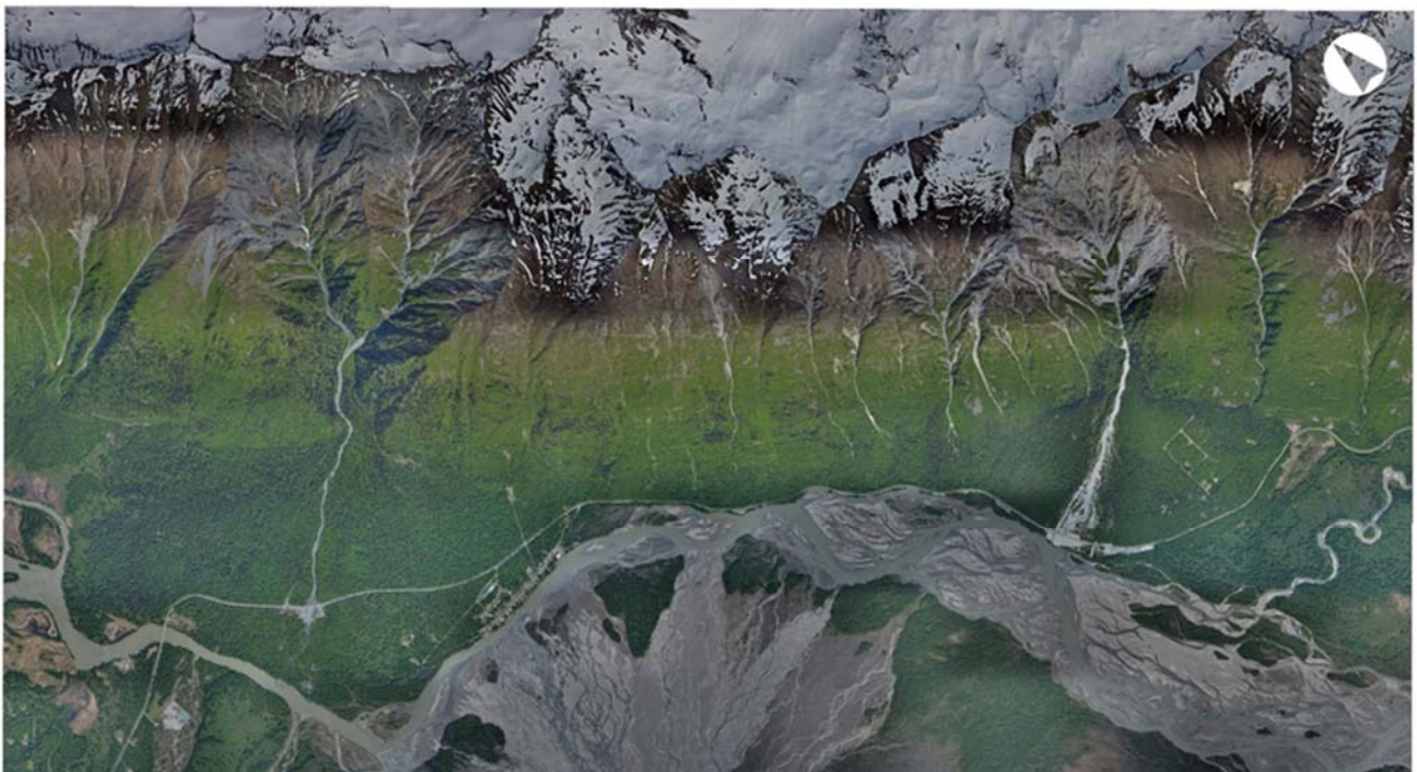
Figure 1. Orthoimage of the west slope of the Takshanuk Mountains and the Chilkat River valley. Debris flow channels can be seen at MP 19 and MP 23 along the Haines Highway north of Haines, Alaska.
