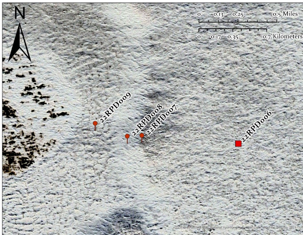
Figure 3. Location of the weather tower (22RPD006) and nodes (22RPD007, 22RPD008, 22RPD009) overlain on visible color imagery, captured by Maxar Technologies Inc. on March 20, 2021, and hosted by Google Earth Pro V. 7.3.6 accessed on December 6, 2022. This figure demonstrates how each node can measure a variety of depths in the snowpack across a relatively small area: 22RPD007 is located on wind-scoured terrain,
