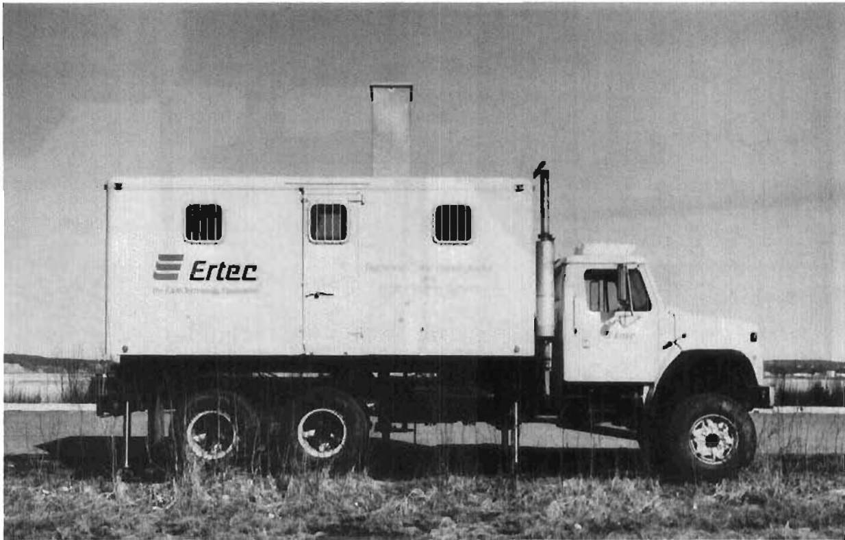
Figure 6. Electric-cone-penetration-test laboratory truck with hydraulic jacks extended before initiating sounding (1982).
