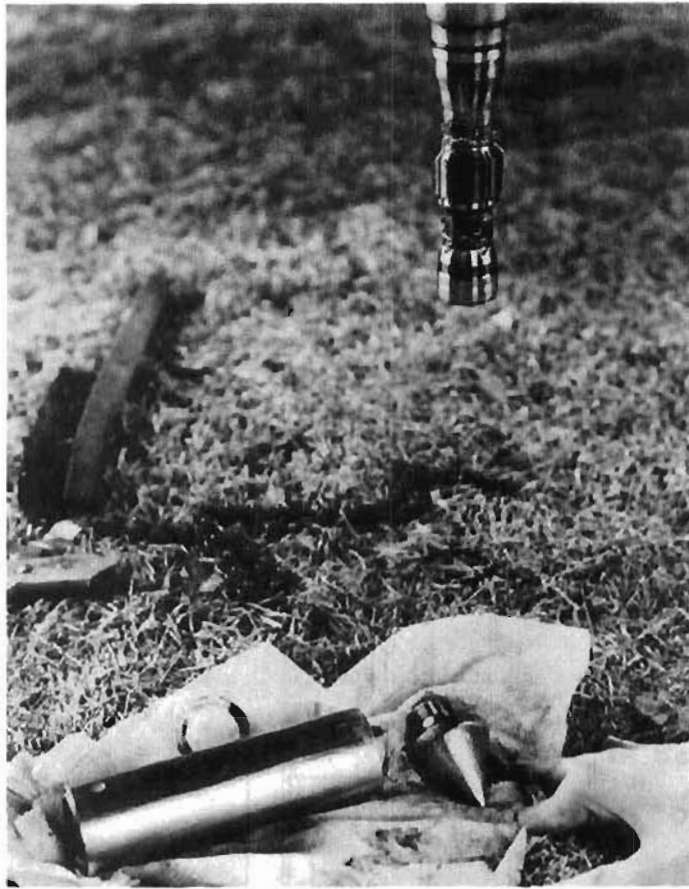
Figure 8. Cone-penetration-test probe with disassembled conical tip and friction sleeve (1982).
