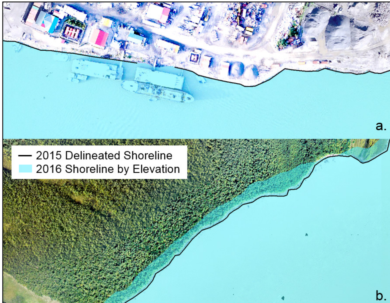
Figure 4. Differences in the visually-delineated shoreline from 2015 and elevation-extracted shoreline from 2016 at (a) a location expected to be stable, and (b) a location with observed erosion between 1950 and 2015. Base imagery is the 2015 orthoimage.
