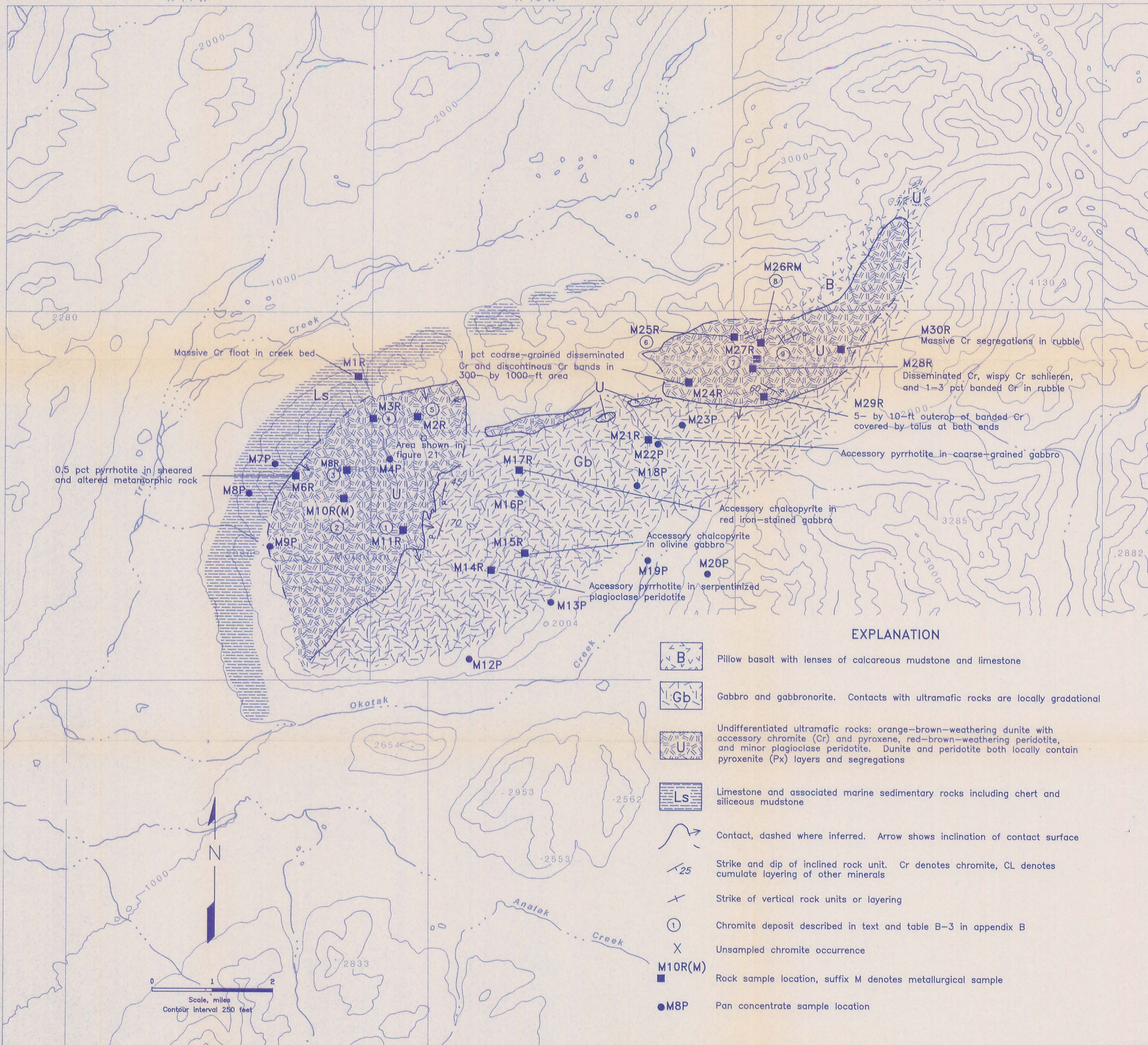
Figure 19. - Geologic map of Misheguk Mountain, showing chromite occurrences, deposits, and sample locations.
