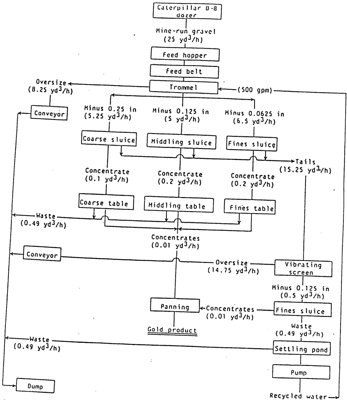
FIGURE 1. - Sample flow sheet, table plant.
