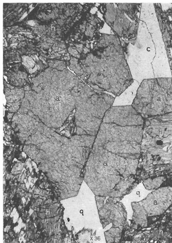
THIN SECTION OF DIOPSIDE-HEDENBERGITE AND TWINNED ANDRADITE IN CRYSTALLINE LIMESTONE. Diopside-hedenbergite (h), andradite (a), and quartz (q) replace the calcite (c). A, Ordinary light; B, Crossed nicols.
