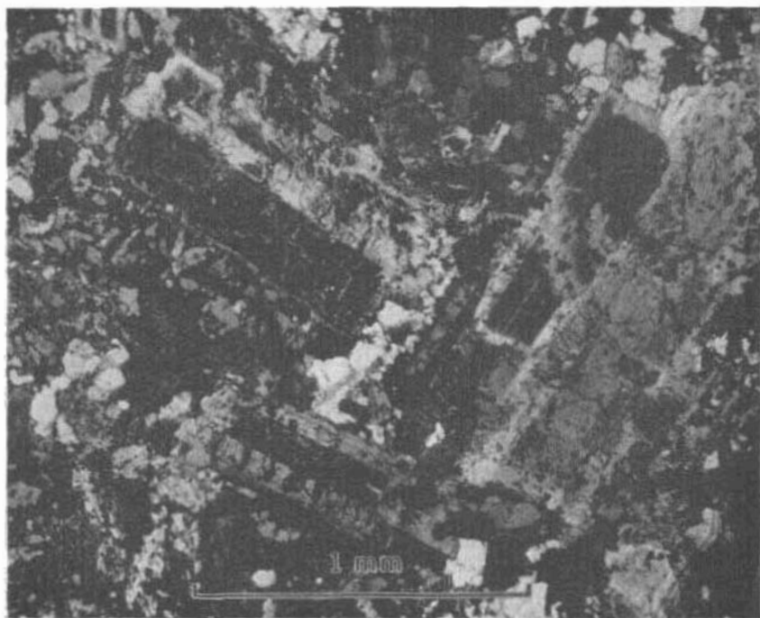
Photomicrograph of plagioclase crystals veined and corroded by orthoclase in altered quartz diorite (specimen no. 47AB:39) bordering granophyre dikes. Crossed nicols.
