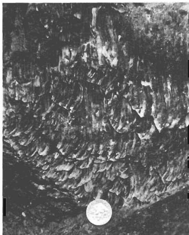
Figure 3. Slickensided high-angle fault surface with curved fibrous slickenlines. Missing block (where photographer was standing) moved down with respect to preserved block. Youngest part of a given slickenline is immediately adjacent to step where it ends. Coin is 17 mm across.
