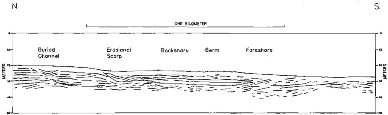
Figure 2. Line drawing of seismic profile across the 24-m beach from the survey conducted in 1976 by the U.S. Geological Survey. The beach deposits are probably 5 to 6 m thick at the berm and nearly 1 km wide.
