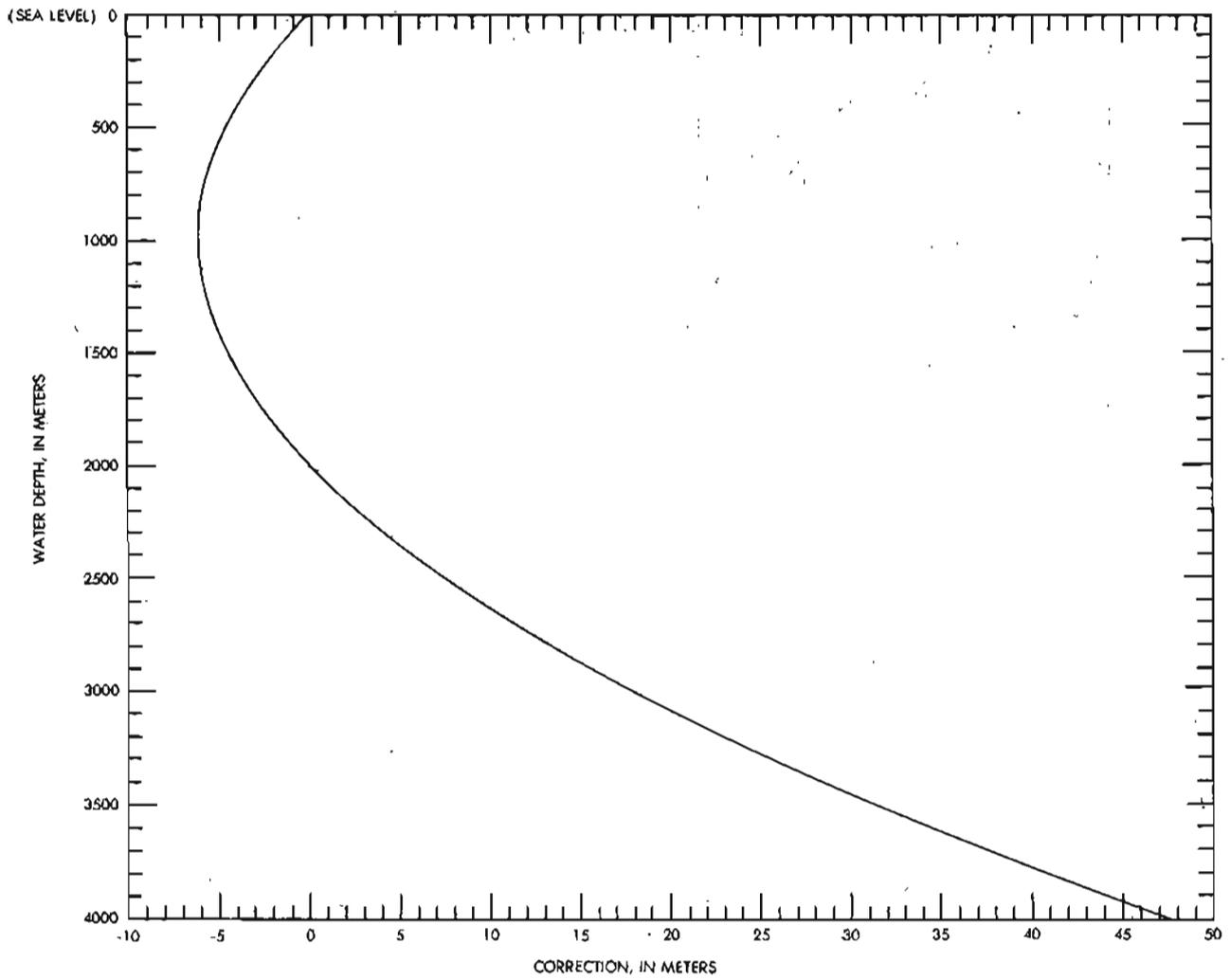
FIGURE 4. Correction factors to be added to the isobaths of the bathymetric map to obtain water depths according to the constantly increasing water velocity model of curve B, figure 3.
