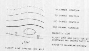
FLIGHT ALTITUDE NOMINALLY 1000 FEET ABOVE GROUND REGIONAL MAGNETIC FIELD SHEET CENTER 56,226 GAMMAS REGIONAL FIELD REMOVED. THE FIELD INCREASES
