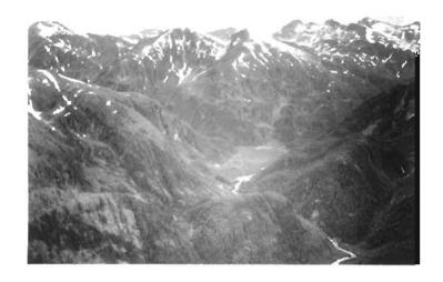
Figure 3. Aerial view of part of Carlson Creek basin looking upstream (west) from a point over the mouth of Carlson Creek. Dam site is in gorge cut through ridge in foreground. Trend of creek at the dam site and parallel gullies on the ridge in foreground define prominent northeast-trending joint set. Creek in lower right corner of picture defines trend of the foliation. Flat-floored basin above the dam site is an alluvium-filled lake.
