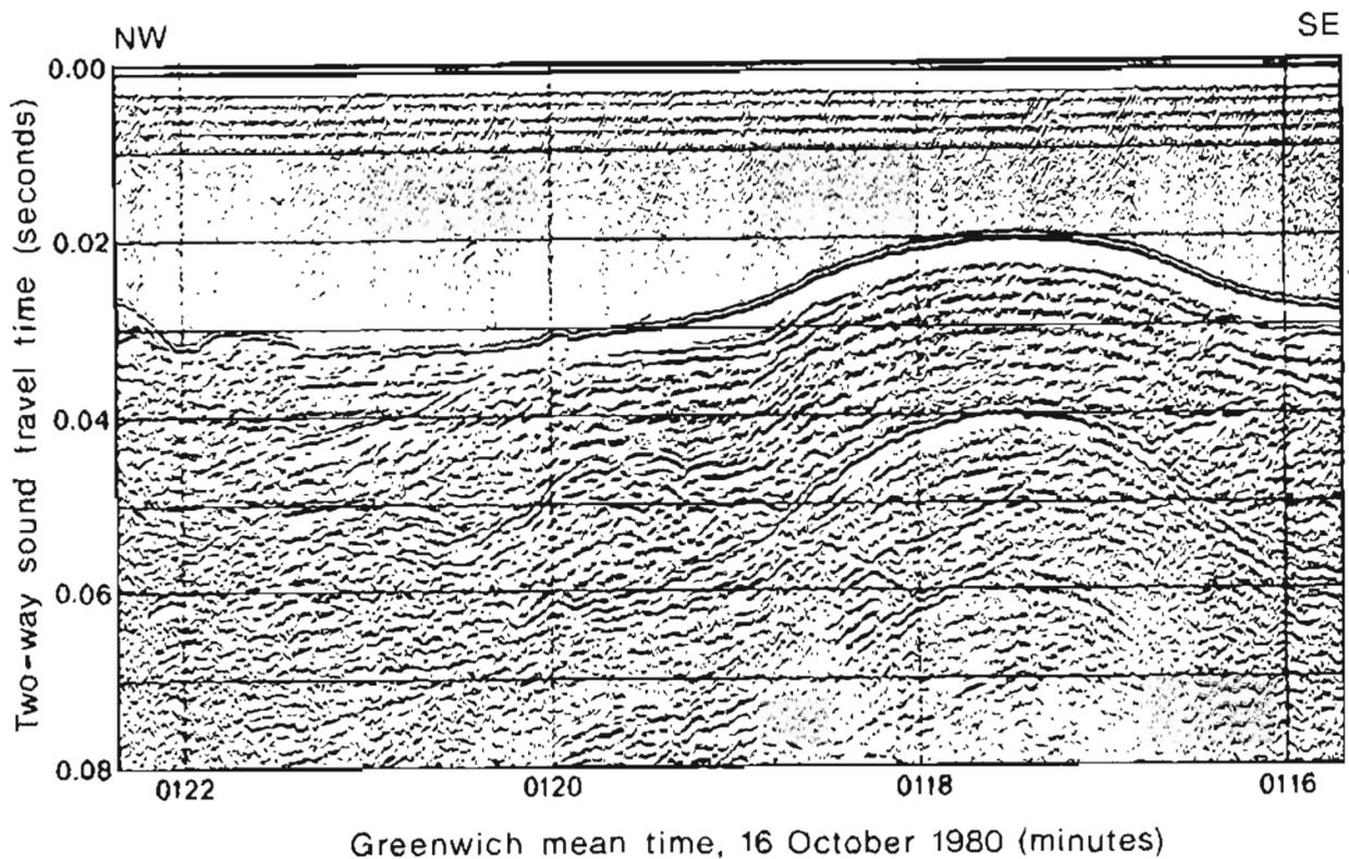
Figure 4. Nearshore half of the 1-kHz subbottom profile along trackline 30, perpendicular to the shoreline and approximately off the middle of the Pillar Mountain landslide. The distance between sea level and the crest of the anticlinal ridge is 15 meters, giving a vertical exaggeration of 3.9 times.
