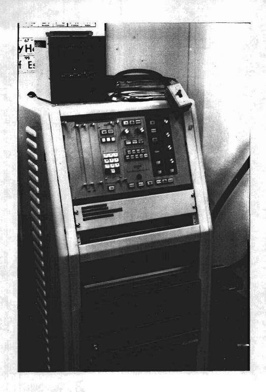
Figure 6. EDAX 707B energy dispersive X-ray analyzer used in routine composition analyses of mineral grains viewed by the linked SEM system.
