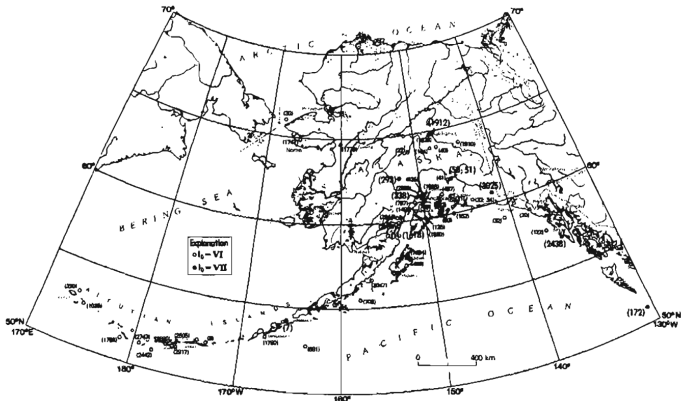
Figure 2a.—Maximum intensity ( I_0 ) for earthquakes which have occurred from 1899 through 1981 in Alaska with I_0 = VI (○), and I_0 = VII (●). The earthquake number for each epicenter is shown in parentheses. Modified-Stereographic Conformal Projection. (From Brockman and others, 1987.)
