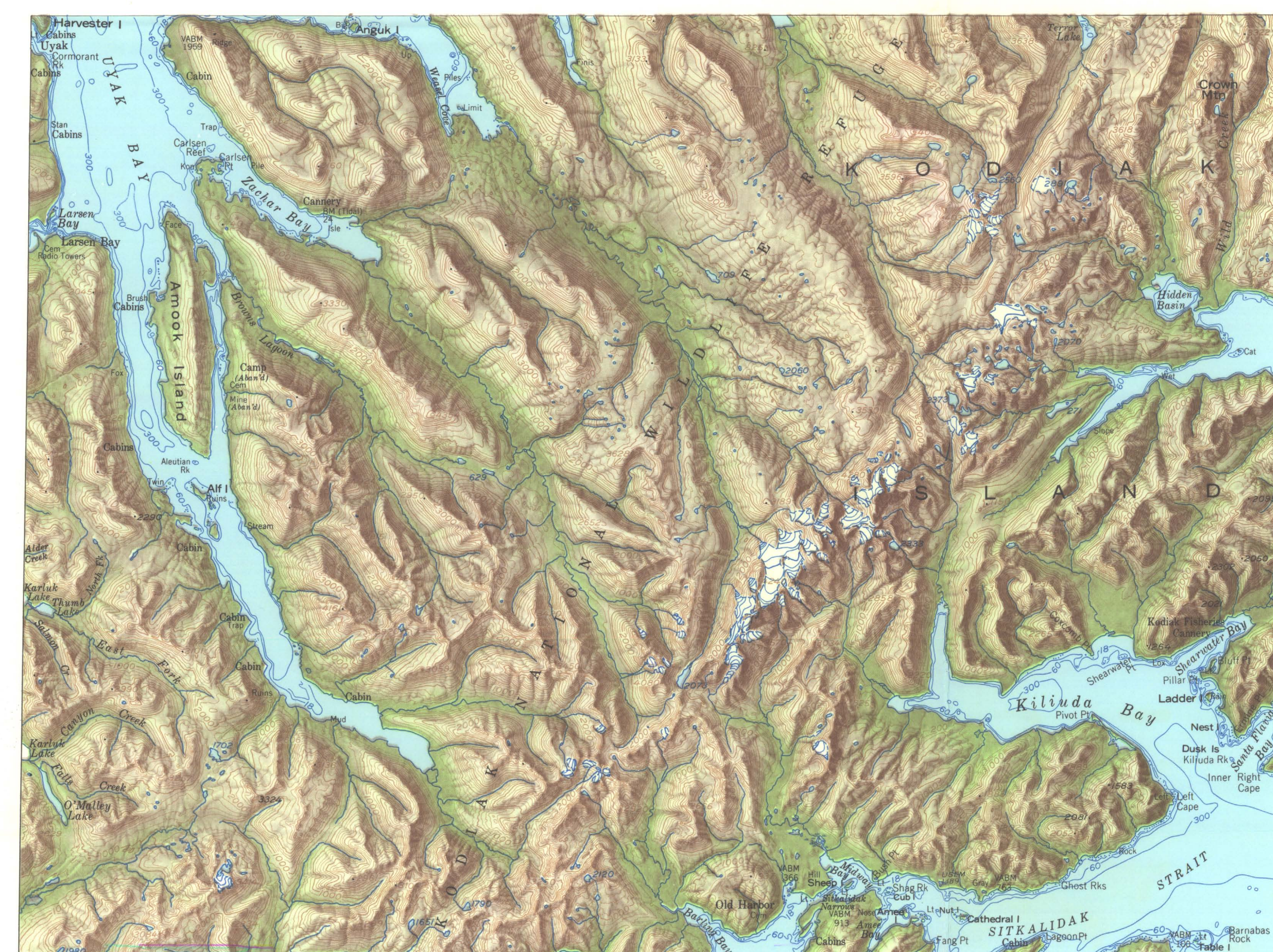
FIGURE 7. CENTRAL PART OF THE KODIAK MOUNTAINS. THE RUGGED NORTHEAST-TENDING DIVIDE IS ON A GRANITIC BATHOLITH. NORTH-EAST-TENDING VALLEYS ON THE EAST COAST ARE UNDERLAIN BY DOWN-FAULTED BODIES OF SOFT TERTIARY ROCKS. THE REMAINDER OF THE AREA IS UNDERLAIN BY GRAYWACKE AND ARGILLITE. KODIAK QUADRANGLE. SCALE 1:250,000. CONTOUR INTERVAL 200 FT.
