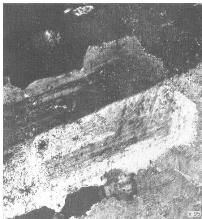
FIGURE 6.—Plagioclase replaced by late orthoclase, with Carlsbad twin boundary retained in orthoclase, Magnetite Cliff, Jumbo basin, Alaska. Crossed nicols.
