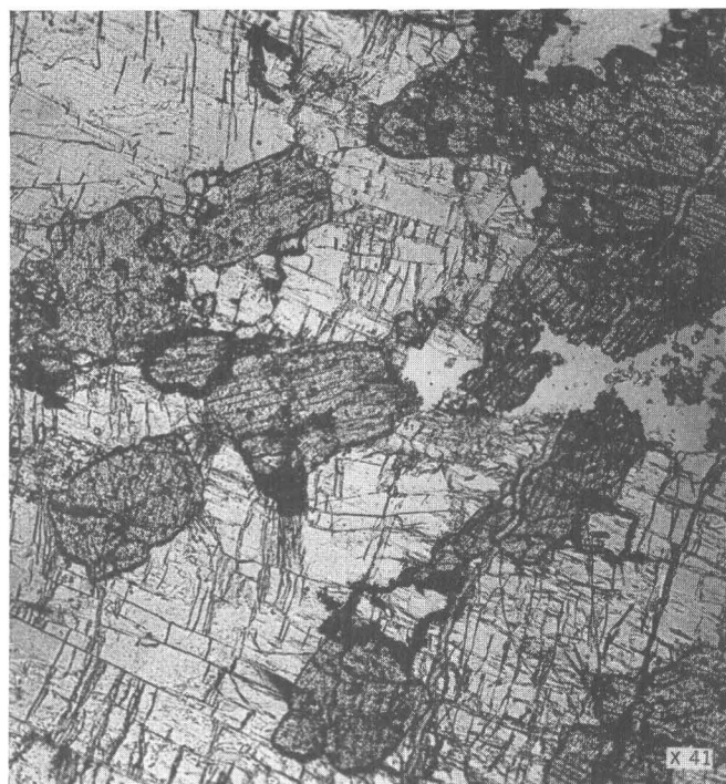
FIGURE 32.—Replaced gabbro, showing coarsely crystalline scapolite, pseudopoikilitically including diopside, Jumbo mine, Alaska.
