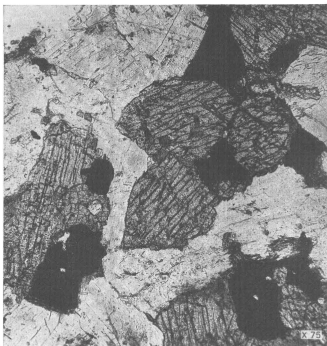
FIGURE 8.—Magnetite preferentially replacing diopside in gabbro, Jumbo mine, Alaska. Plane light.
