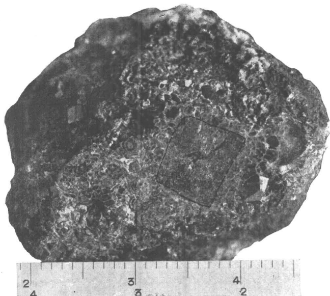
FIGURE 25.—Uralitized diopside crystal, partially replaced and surrounded by garnet. Jumbo mine, Alaska.
