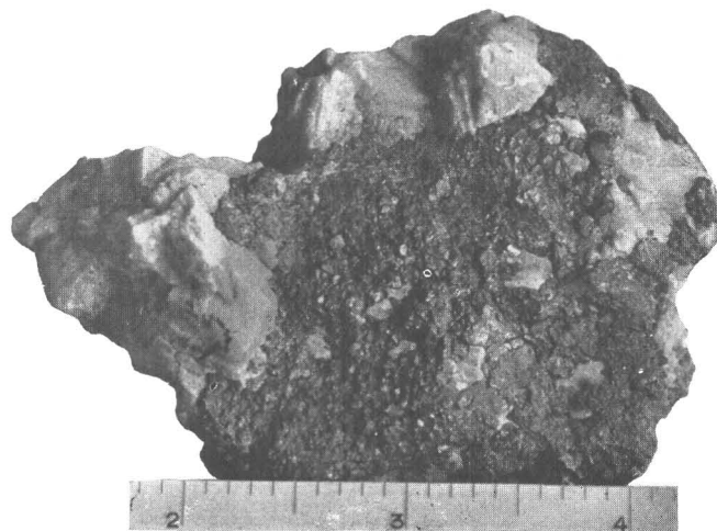
FIGURE 23.—Magnetite-diopside intergrowths replacing marble, upper magnetite bodies, Jumbo basin, Alaska.
