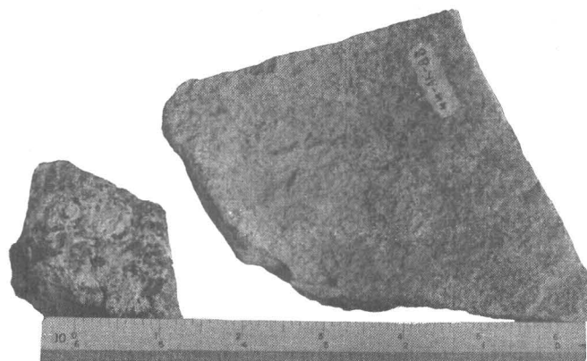
FIGURE 33.—Gradation in altered augite monzonite from (right) fresh rock to (center) sericitized and chloritized rock to (left) rock composed of coarsely crystalline epidote and albite, Jumbo mine, Alaska.
