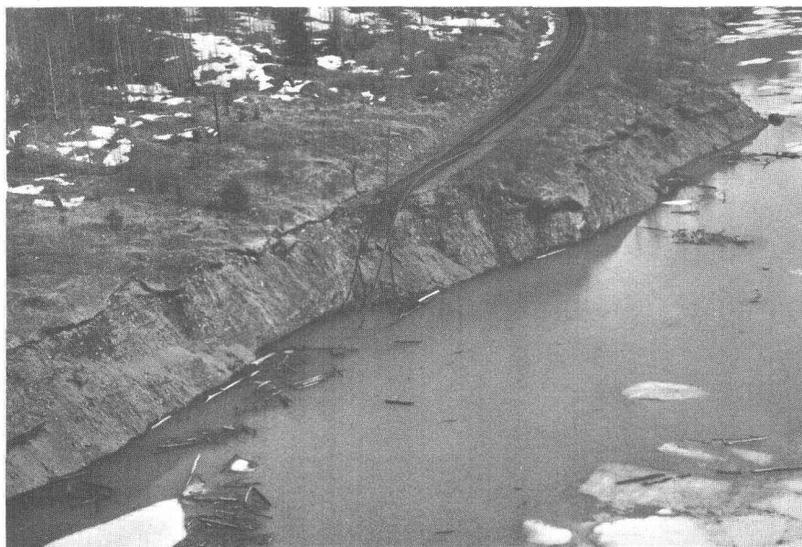
19.—Scarps along the front of Rocky Creek delta produced by many small slump-type slides. The gently dipping coarse sediment is clearly visible. With the exception of the sandy lens at left, most of the sediment is dry.
