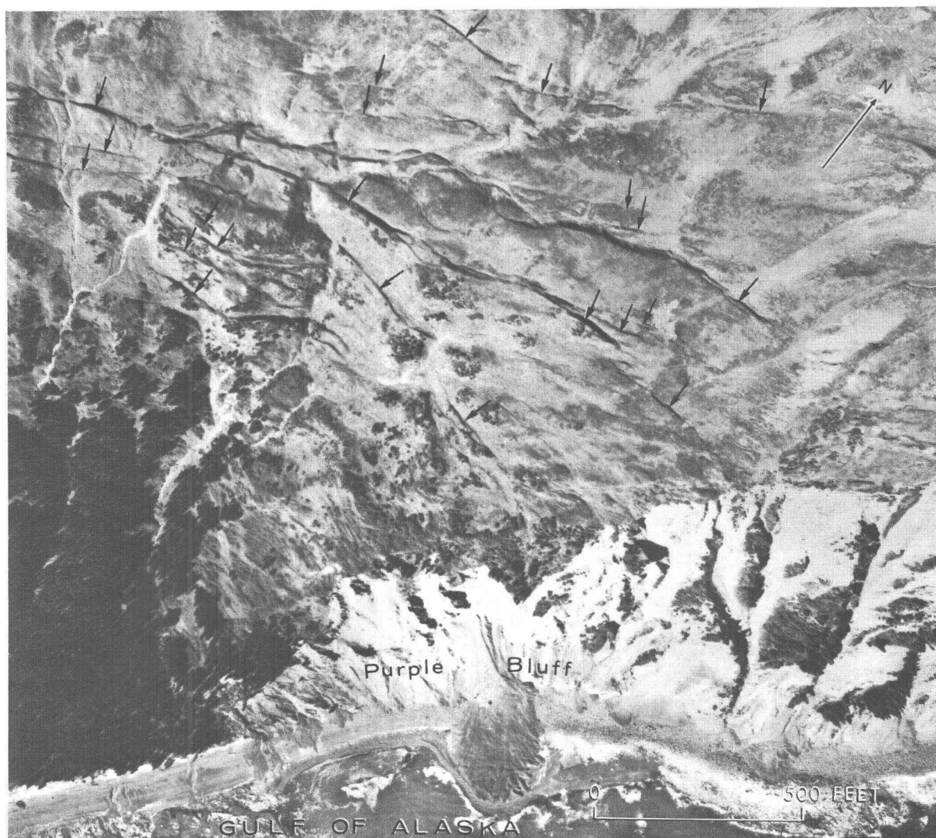
24.—Vertical aerial photograph in the vicinity of Purple Bluff showing conspicuous lineaments (arrows) along the inferred northeastward extension of the Patton Bay fault. Renewed displacement occurred on some of these lineaments after the 1964 earthquake. A large earthquake-induced landslide may be seen at the base of the high bluff at bottom center. Photograph by U.S. Coast and Geodetic Survey, August 25, 1964.
