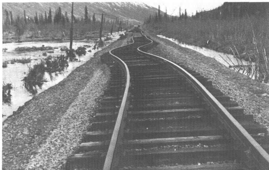
98.—Lateral kinks in the tracks, at mile 35 on Hunter Flats, which may have resulted from longitudinal compression of the embankment.
