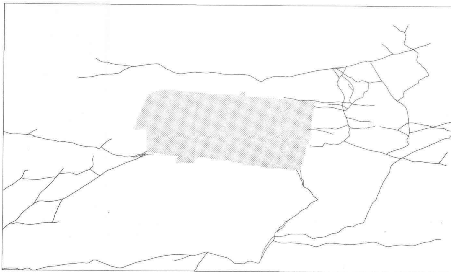
47.—Photograph and sketch of ground cracks localized at the corners of the U.S. Forest Service crew house on Portage Creek flood plain. Cracks broke the foundation and the building was moved to a new foundation. Photograph by Arthur Kennedy, U.S. Forest Service, Anchorage.
