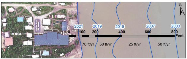
**Figure 1.** Kuskokwim River shorelines (blue) in relation to the school. The image is from the June 29, 2021 drone survey. The average erosion rate from 2003 to 2021 is 40 feet per year. Recent rates are 50 to 70 feet per year. The school is 79 feet from the bank and about 260 feet long.
