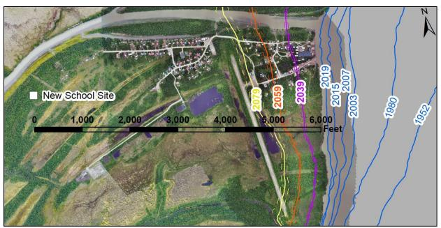
**Figure 2.** Forecast erosion from 2019 to 2079 based on the weighted linear regression rate of shoreline change from 1952 to 2019. The June 29, 2021 image is shown (darker image) along with the 2015 image (lighter image to the left) in areas beyond the newest image's boundary. Forecast uncertainty is at a 90 percent confidence interval.
