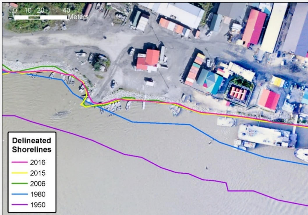
Figure 2: Emmonak delineated shorelines, including shoreline derived from 2016 Lidar data. Image courtesy of J. Overbeck, State of Alaska DGGS.
