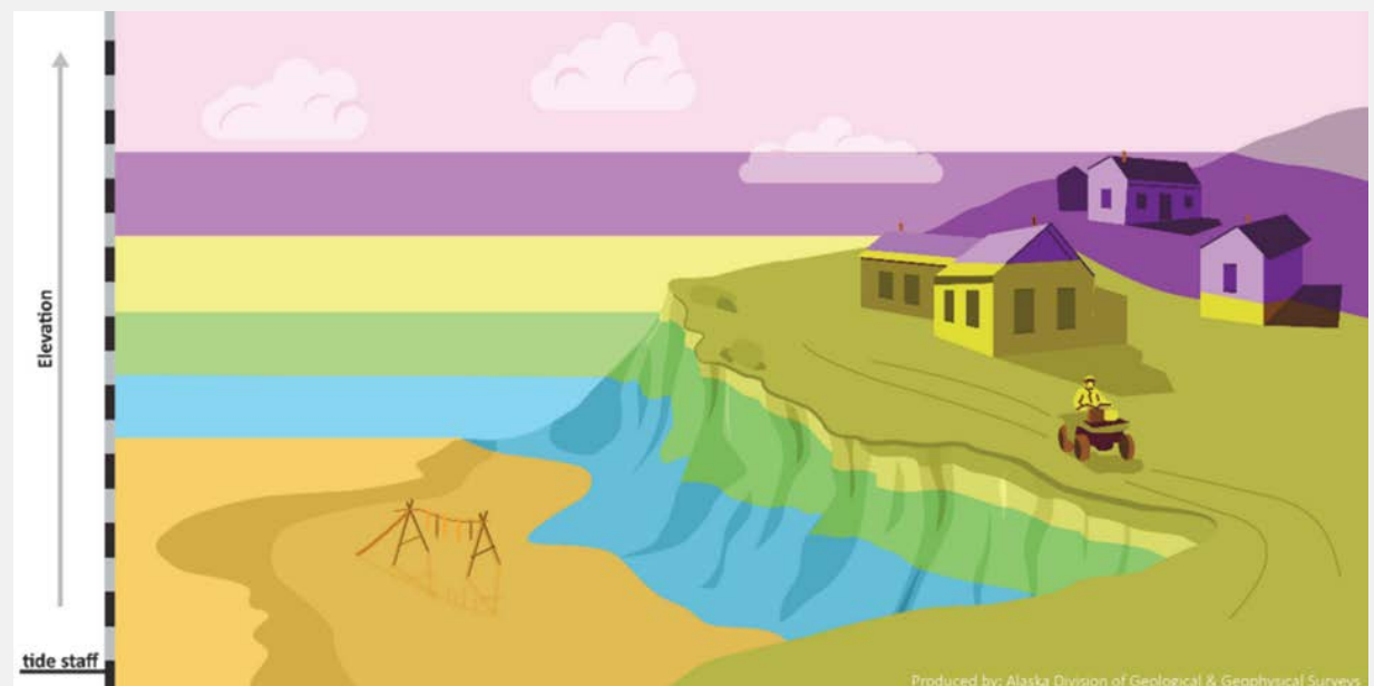
Figure 9: Schematic of color-indexed elevations as they relate to local topography, beaches, and coastal infrastructure. Image courtesy of J. Overbeck, State of Alaska DGGs.
