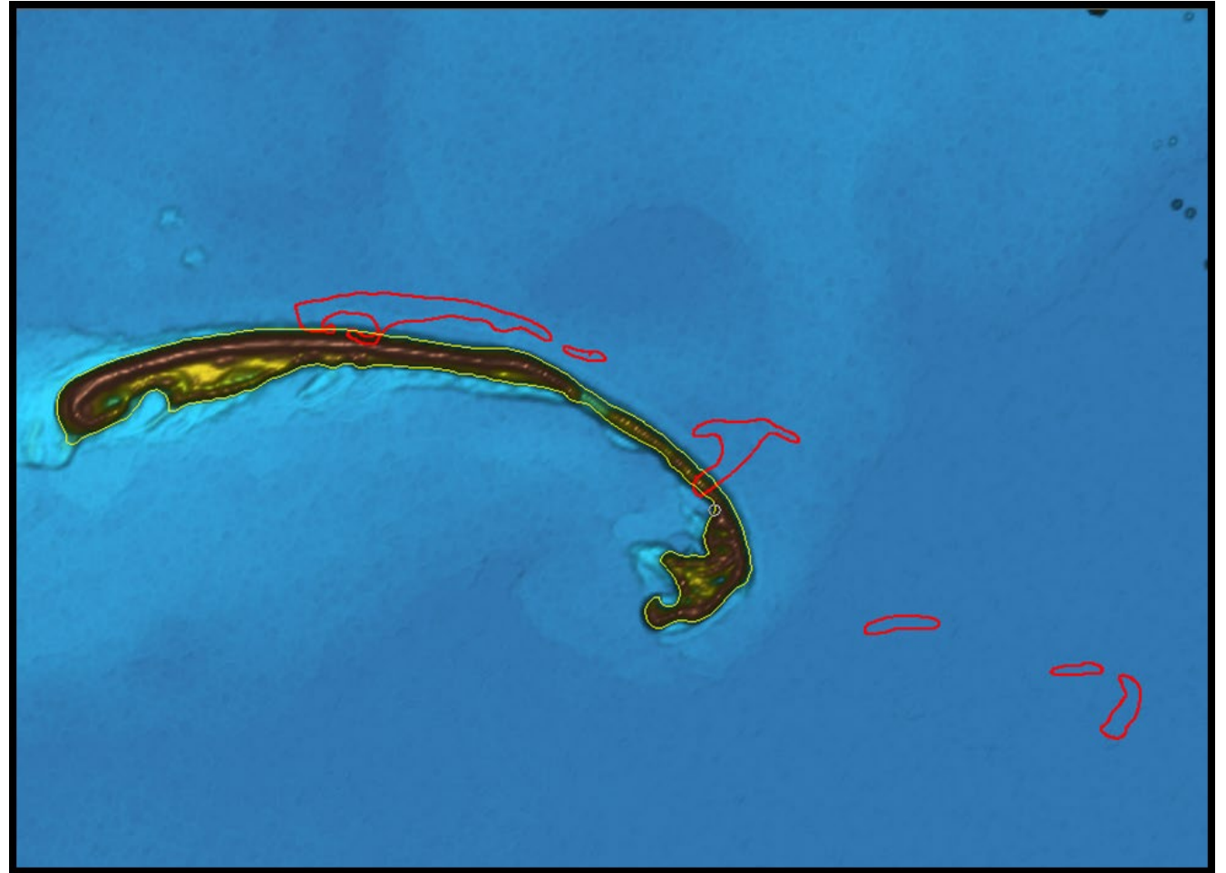
Reindeer Island, Prudhoe Bay, Alaska Difference between 1955 nautical chart (red) and a recent satellite image
