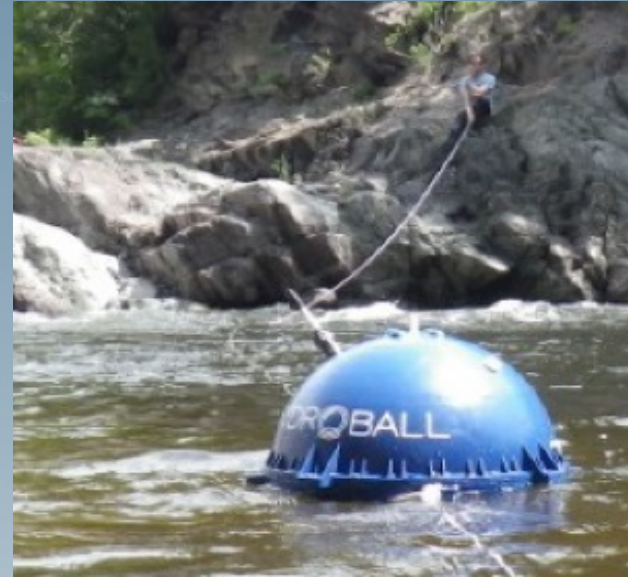
Hydroball buoy with GNSS and multibeam sonar
