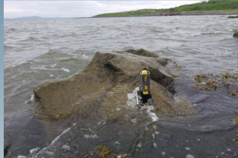
Non-vented pressure tide gauges have some advantages over vented gauges
