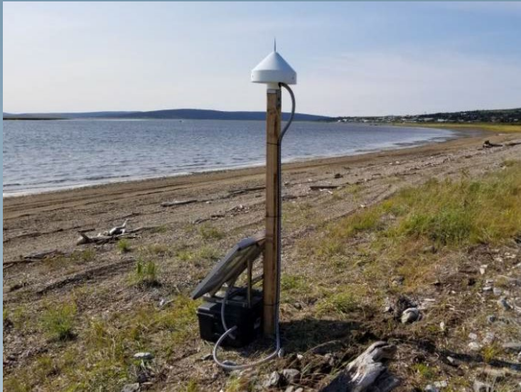
GNSS-Reflectometry determines height of the antenna above a reflected surface
