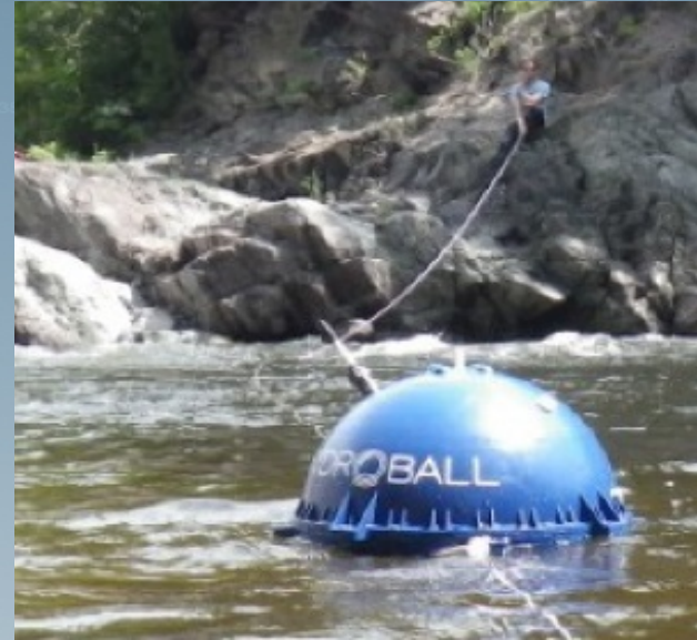
Hydroball buoy with GNSS and multibeam sonar
