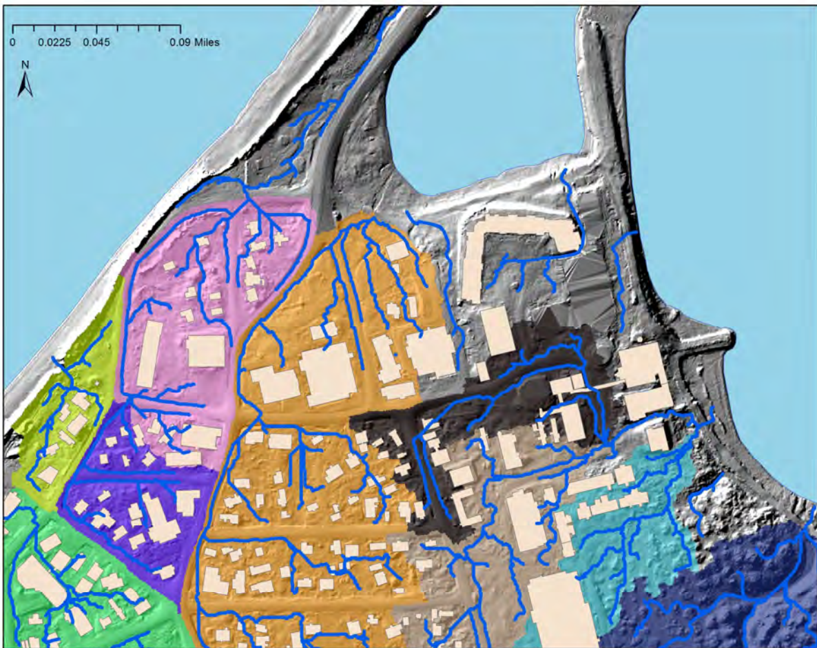
Figure 7. Basins, Water Flow Lines, and Structures
