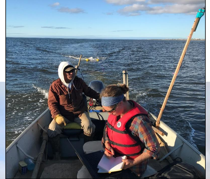
Boat operator with the Olgoonik Corporation Blair Patkotak and Jaci Overbeck, DGGs, tow the hydroball for single-beam bathymetry collection.
