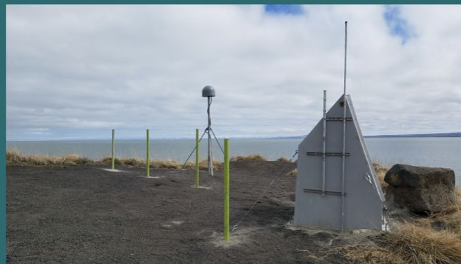
Stebbins/St. Michaels GNSS-R Station, AOS/UNAVCO (photo courtesy UNAVCO)
