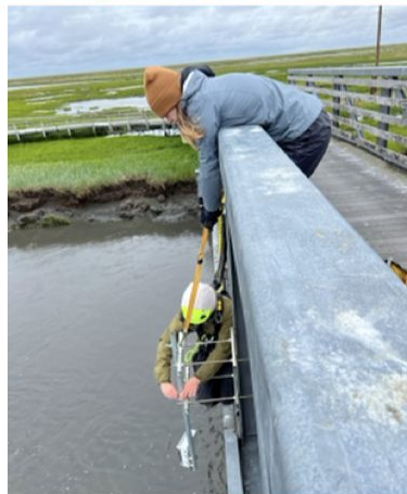
AKDNR-DGGS staff re-install an iGage® at Kwigillingok.
