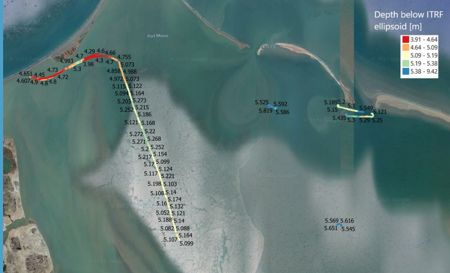
Elson Lagoon bathymetry, surveyed on August 31, 2021 with a hydroball
