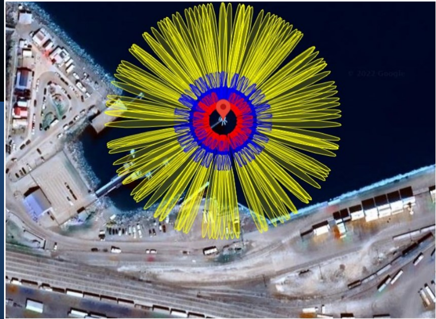
Option 1 is well suited for GNSS-R because of its broad water visibility.
