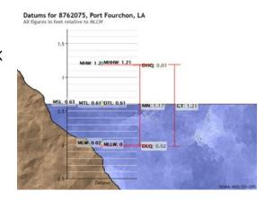
Image caption: This graphic shows currently accepted tidal datums at the Port Fourchon water level station in LA. Heights depicted will change when the new NTDE is launched.
