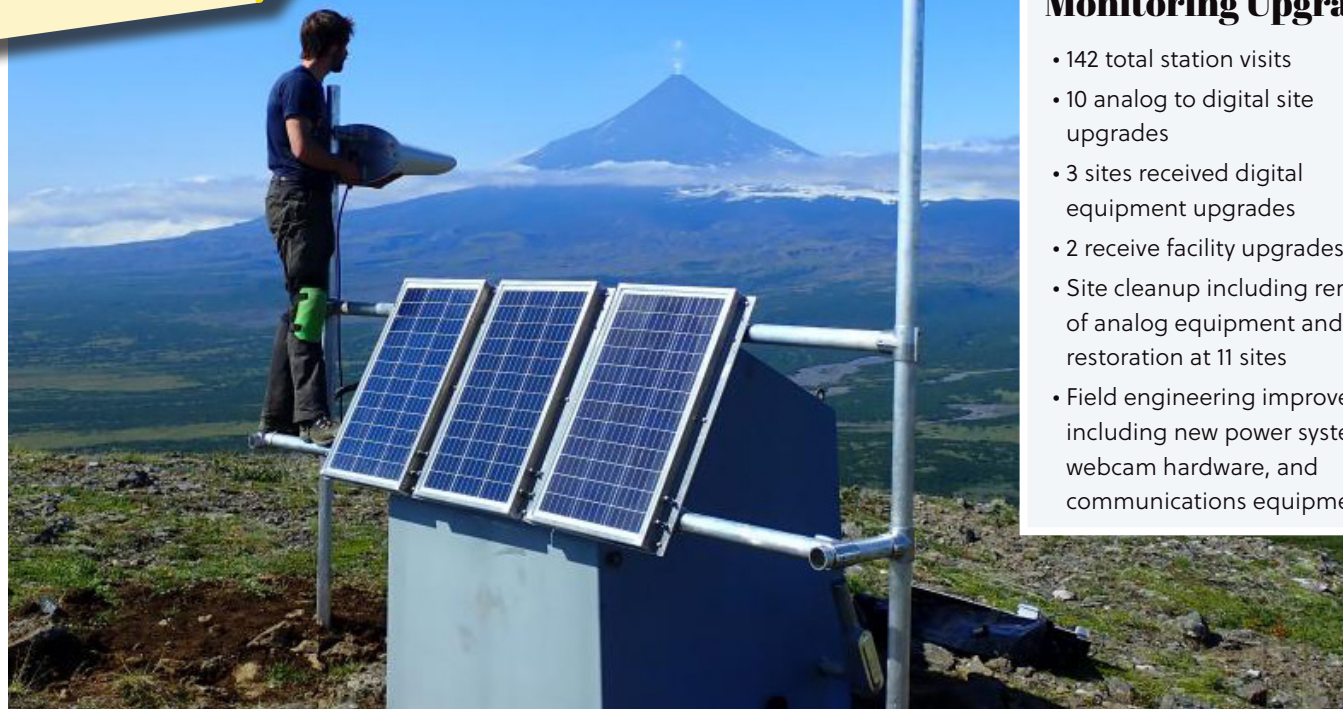
Dane Ketner (USGS/AVO) orients a radio antenna toward a site near Shishaldin Volcano, August 20, 2020. View from SE at geophysical site BRPK. Shishaldin Volcano is emitting a gas plume and the edifice is covered with debris from 2019–2020 eruption. Photo: Allan Lerner.
