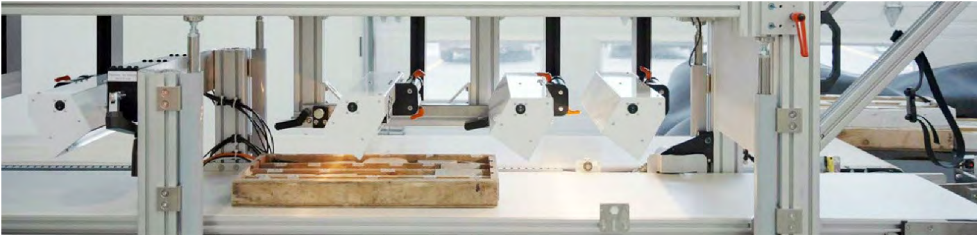
Below. Hyperspectral scanning instrument imaging a mineral core box. Photo. Photon etc, 2022.
