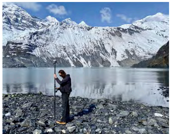
DGGs scientist Ronnie Daanen collects ground control points for a lidar survey during 2022.
