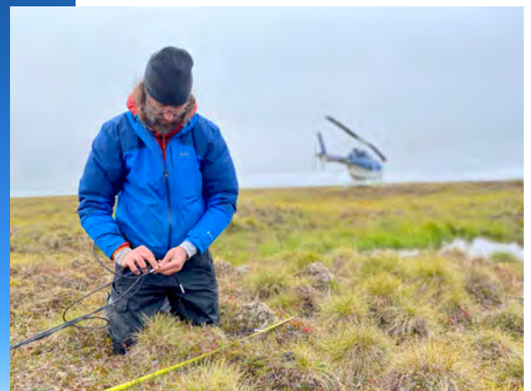
Left. A helicopter transports equipment necessary to collect hydrology data on the North Slope. Right. DGGs hydrologist Ronnie Daanen installs soil temperature sensors on the North Slope as part of the ASTAR project.
