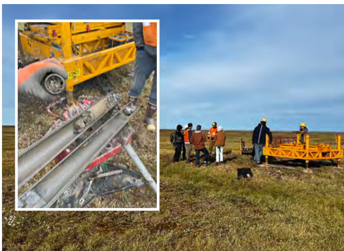
A helicopter-supported drill rig was used during fieldwork by partner agency AKDOT&PF to collect surface and near-surface samples as part of the ASTAR project.
